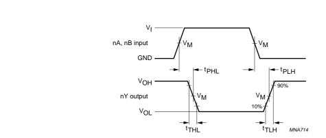
For 74HC2G00:  $V_M$  = 50%;  $V_I$  = GND to  $V_{CC}$ . For 74HCT2G00:  $V_M$  = 1.3 V;  $V_I$  = GND to 3.0 V.
